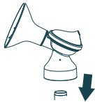
Pull the membrane out of the connector
